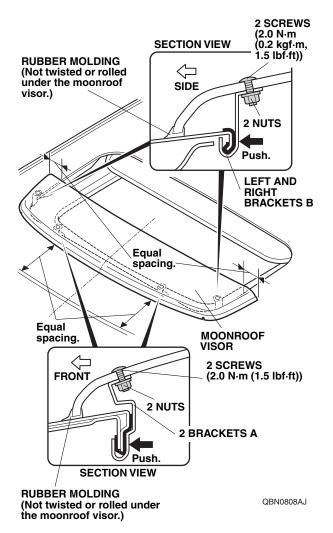
Tighten two screws and two nuts on the front of the vehicle first, then tighten two screws and two nuts on each side. Tighten while applying pressure so that there is no gap between the roof panel and the brackets A and B. Torque the screws to 2.0 N·m (1.5 lbf·ft). 14. Remove the shop towels inserted in step 2. Remove the IMPORTANT INFORMATION label.
