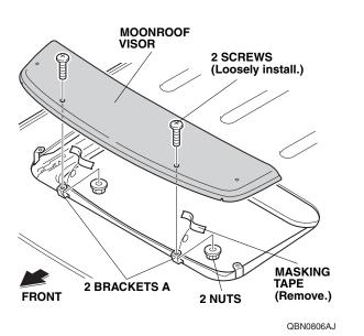
11. Loosely install the moonroof visor to the brackets B with two screws and two nuts. Remove the strips of masking tape from the brackets B.
