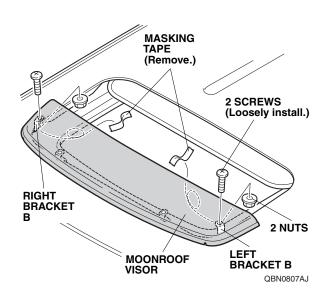
12. Position the moonroof visor with equal spacing in the front and on the sides. Check that the rubber molding is not twisted or rolled under the moonroof visor.
